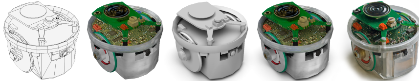
Fig. 2: Development steps for the creation of the e-puck model. Left to right: wireframe of the model; texture map; radiosity map; texture and radiosity maps combined; photo of the real robot.
