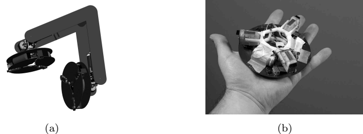
Fig. 6. (a) A preview of the future climbing robot Tremo . (b) The developed magnetic anchor for TREMO with 3 emedded MSDs .
