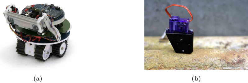
Fig. 5. (a) The MarXbot robot with the magnetic gripper module. (b) The docking station developed for a flying quadrator.
