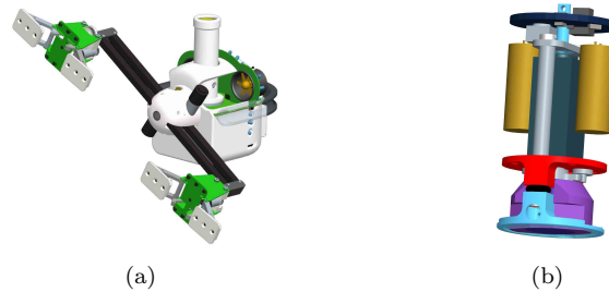
Fig. 4. (a) An overview of the Hand-Bot . (b) The magnetic grapnel with embedded MSD .
