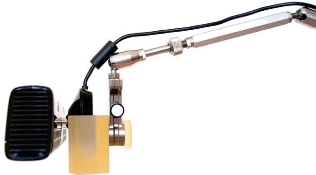
Figure 3.2: Lateral view of the Kinect camera mounted on the holder and the suspension arm
