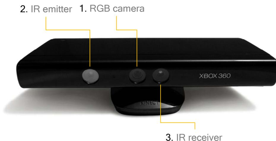
Figure 2.1: Core components of the Microsoft Kinect
