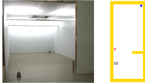
Fig. 21 Arena used in the real robot experiments: photograph (left) and as reproduced in simulation (right). The photograph was taken from the position of the camera icon in the right image. In this image, the circle and the disk symbols indicate respectively the position of food and nest robots.
