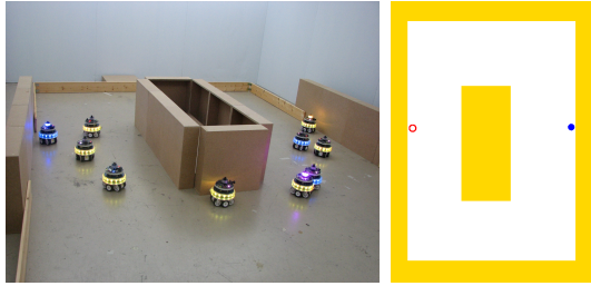
Fig. 23 Arena used in the real robot experiments with obstacle: photograph (left) and as reproduced in simulation (right). The circle and the disk symbols in the right image indicate the position of the food and the nest robots.
