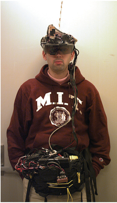
Fig. 2. The vision of wearable computing in the mid 1990s (from [22]). The system comprises a head-worn camera, a see-through head-up display in the goggles, an Internet connection, and an on-body computer.
