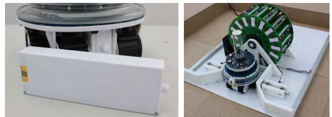
Fig. 2: The battery (left) and the exchange and recharge station (right).
